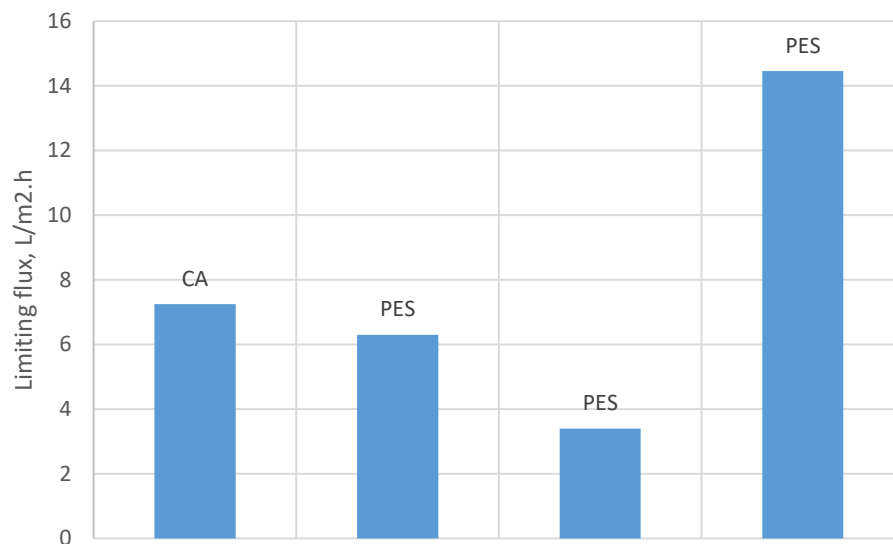
Figure 4.15 Limiting filtration flux for OWE-Tween 80 filtration on CA and three different PES straight membranes
